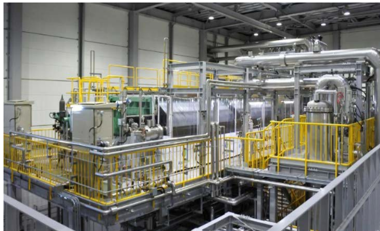
10MW Alkaline Water Electrolysis Fukushima, FH2R
